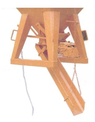
The 1300mm long discharge chute is used in conjunction with the standard TUC quick release fitting to enable concrete to be poured into structures where access is a problem
