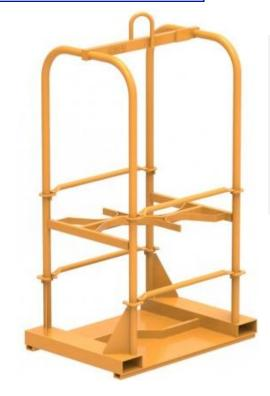
**Presentation:** Two lateral fork pockets allow the bottle rack to be lifted by a forklift. An upper hook has been designed to enable the lifting through cranes, tackles or overhead cranes on forklift. The bottles are held by semi-circle and removable rigid bars.
